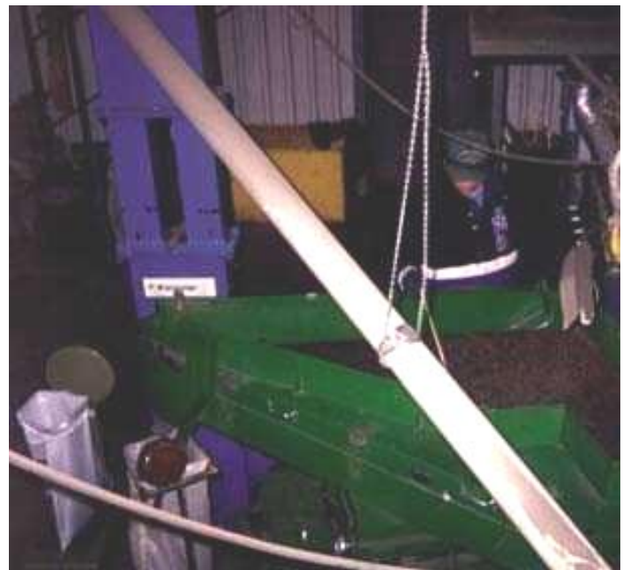
The green machine vibrates to separate pure mânomin from other stuff, then it is bagged (bottom left). The man is doing quality control.
